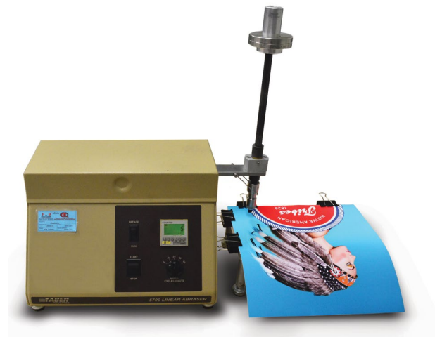
Figure 1 Scratch and abrasion testing are performed using a Taber tester, according to industry-standard test methods. 5
